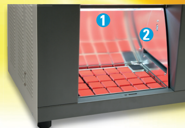
1: Xenon lamp, 2: Light monitor
